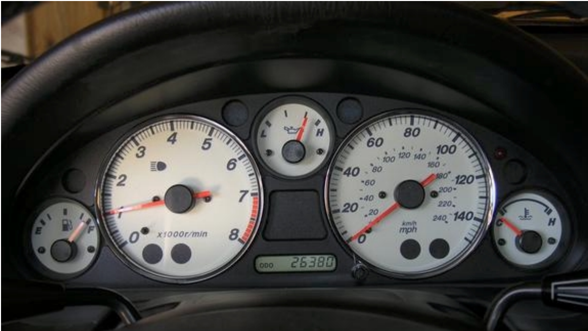
Light off and the gauge showing pressure (engine running)
