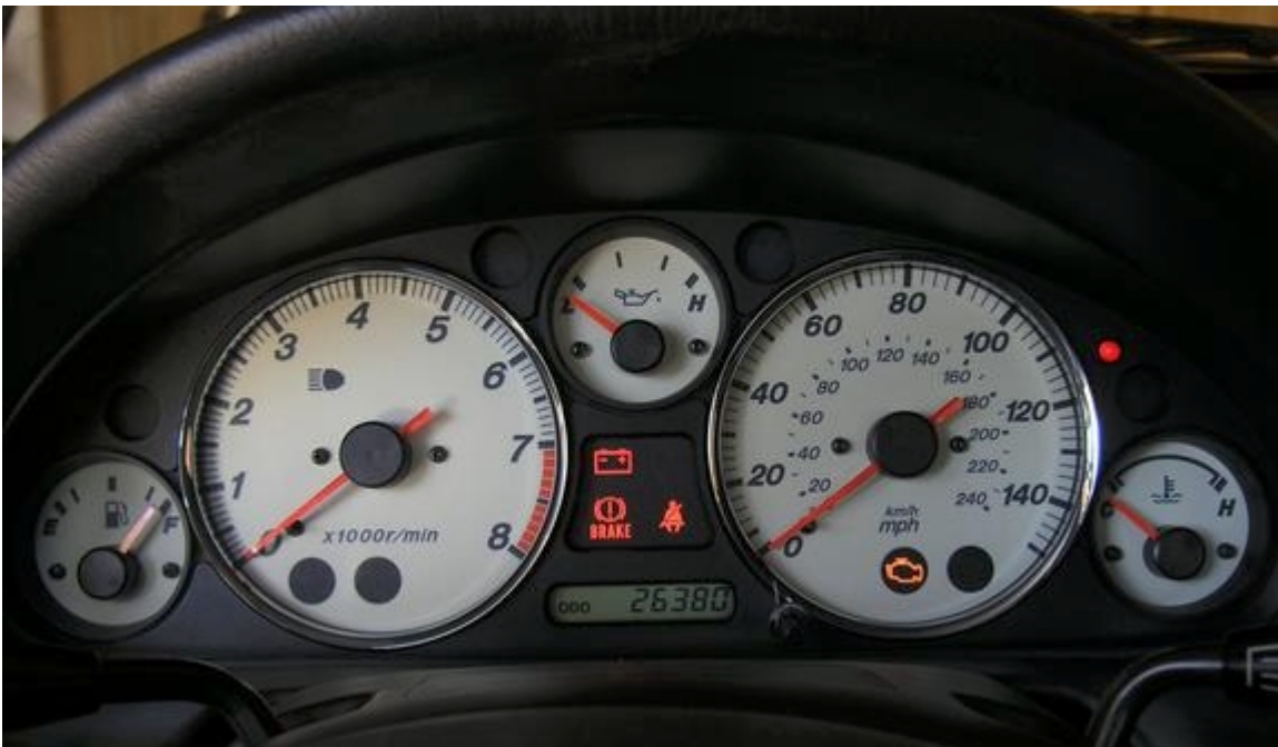
No oil pressure and the light is on (engine off but ignition turned on)
