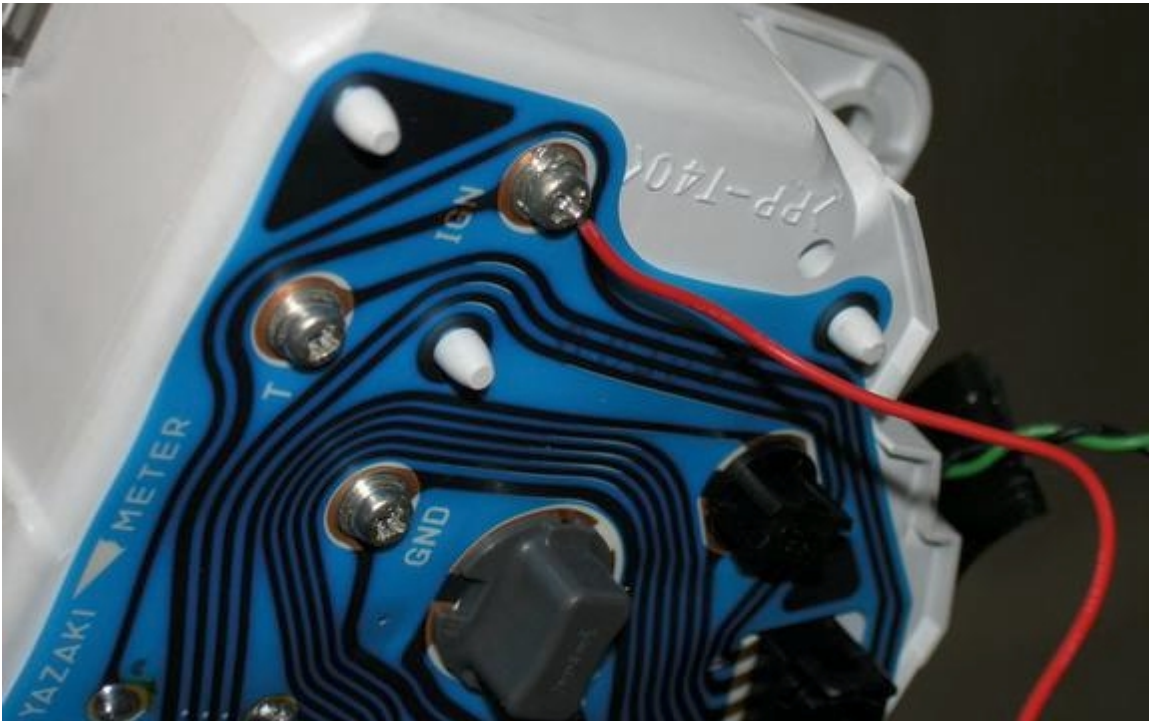
Wire attached to the "IGN" screw on the back of the cluster.
