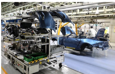
During production, the car is followed by an automatic parts carrier that runs alongside it. All of the components necessary to build the vehicle to a unique specification are contained within it.
