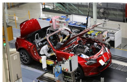
Putting the dashboard in place. Two skilled workers build up the dashboard to the required specification, adding meters and displays, and then mount it in the vehicle as a complete unit.
