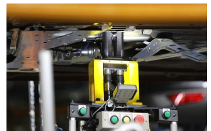
The building station for the PPF, a key feature of the MX-5. A special machine tightens the front and rear bolt sets at the same time to a preset torque value.
