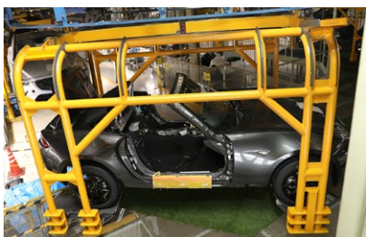
Computers automatically compensate for the variations in wheelbase measurements at turning points in the line, delivering the correct cage to suit the vehicle. This system allows different cars to share the same production line.
